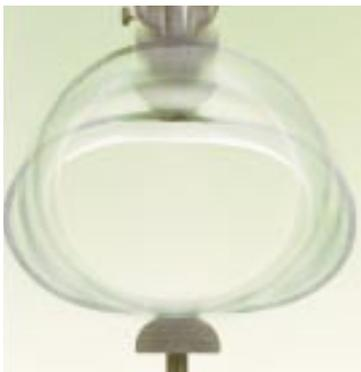
Even after 19,300 N/m test pressure, the Inpipe liner returns to its original shape. That is 10 times more than a normal stiffness test.
